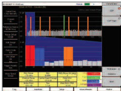
CDMA Code Domain Power measurement display
