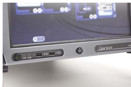
Figure 2 - LXI Class B compliant with IEEE 1588 synchronization of better than 50 ns over Ethernet
