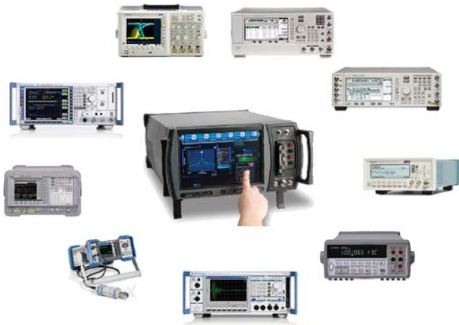
Figure 1: The 7200 takes the place of an entire suite of test equipment
