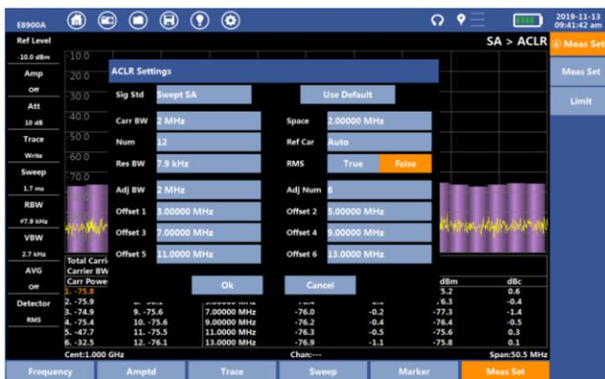
Fig.3-17 measurement setting
