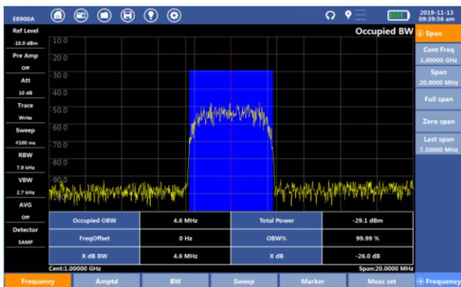
Fig.3-13 Occupied bandwidth
