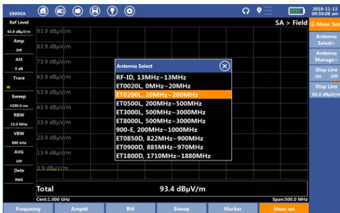
Fig.3-20 Field Strength Antenna List
