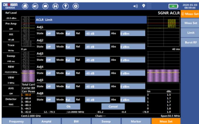
Fig.8-29 5G ACLR Measurement setting
