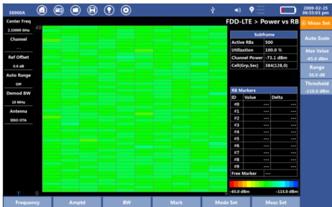
Fig.6-1 Power vs RB measurement
