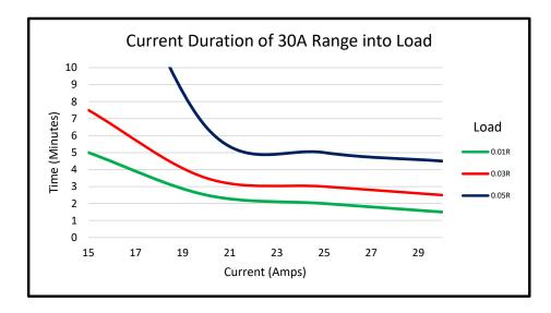
Measurement Conditions : Ambient Temperature 20'C, Mains Voltage 230V, Mains Frequency 50Hz Allow at least 7 minutes 'off' period between current output
