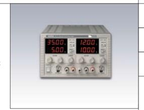
The Xantrex XPF is a new type of bench power supply designed to meet the need for flexibility in the choice of voltage and current. Typically, the maximum voltage and maximum current are not required simultaneously. The PowerFlex design enables higher currents to be generated at lower voltages within an overall power limit envelope. This is achieved by using the latest switch-mode technology.
