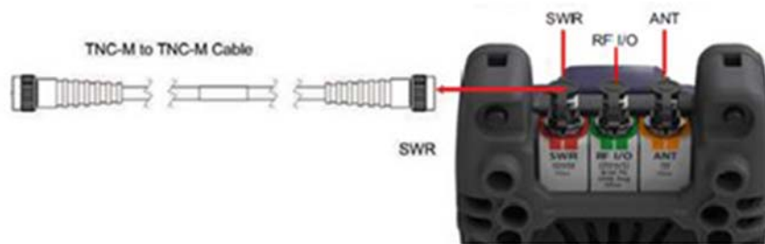
Figure 18: VSWR Calibration Setup Diagram
