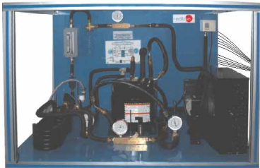
① Unit: THALAC. Air Conditioning Unit (one condenser (water) and one evaporator (air))
