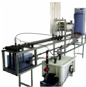
① Unit: EGAC. Water Hammer Unit
