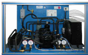
① Unit: THALAC/1. Multiple Compressor Refrigeration Control
