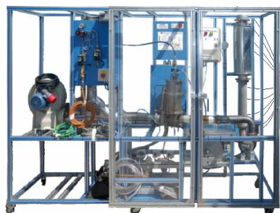
① Unit: TGDEPC. Two-Shaft Gas Turbine/Jet Engine
