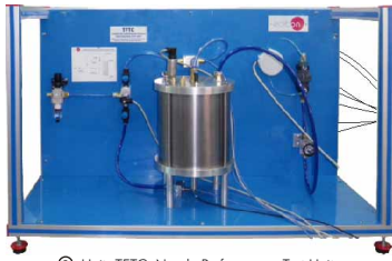
① Unit: TFTC. Nozzle Performance Test Unit
