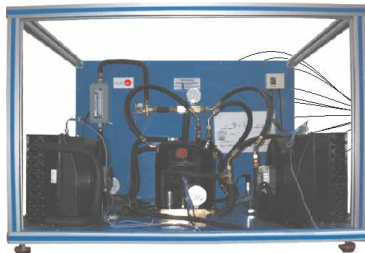
① Unit: THAAAC. Air Conditioning Unit (one condenser (air) and one evaporator (air))
