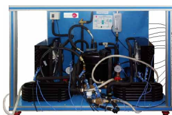
① Unit: THAR22C. Refrigeration and Air Conditioning Unit (two condensers (water and air) and two evaporators (water and air))
