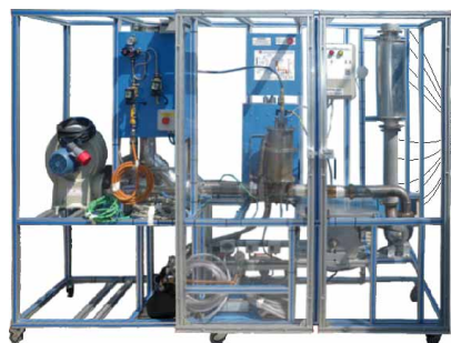
① Unit: TGDEC. Two-Shaft Gas Turbine
