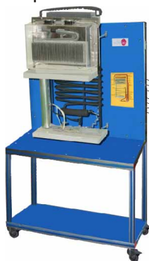
① Unit: TRAC. Absorption Refrigeration Unit
