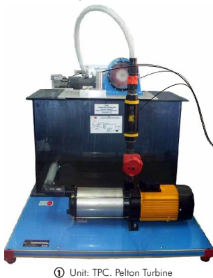
① Unit: TPC. Pelton Turbine
