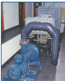
① Unit: TA500-500. Water Tunnel, 500 x 500 mm
