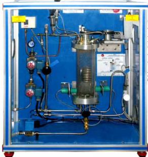
① Unit: TTVC. Steam Turbine
