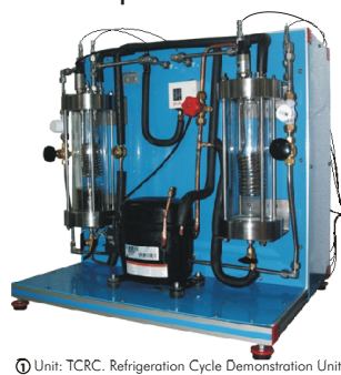
① Unit: TCRC. Refrigeration Cycle Demonstration Unit
