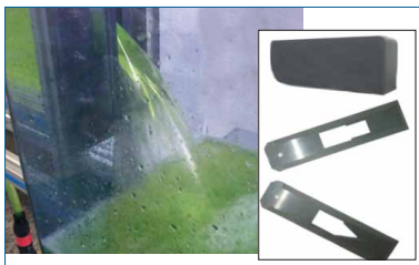
CFVDG. Broad and thin crested weirs
