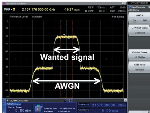
Wanted signal + AWGN signal output from one unit
