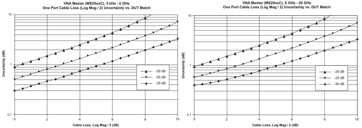
These uncertainty curves show how frequency range, DUT Match, and cable loss impact worst-case uncertainty of round-trip cable loss measurements. The uncertainty curves, separated by frequency range, are shown for DUT Match cable loss conditions of -20 dB, -25 dB, and -30 dB. For DUT Match of 30 dB and cable loss of 4 dB to 5 dB (reflection measurement of 8 dB to 10 dB) the worst-case uncertainties are approximately  $\pm 1$  dB.
