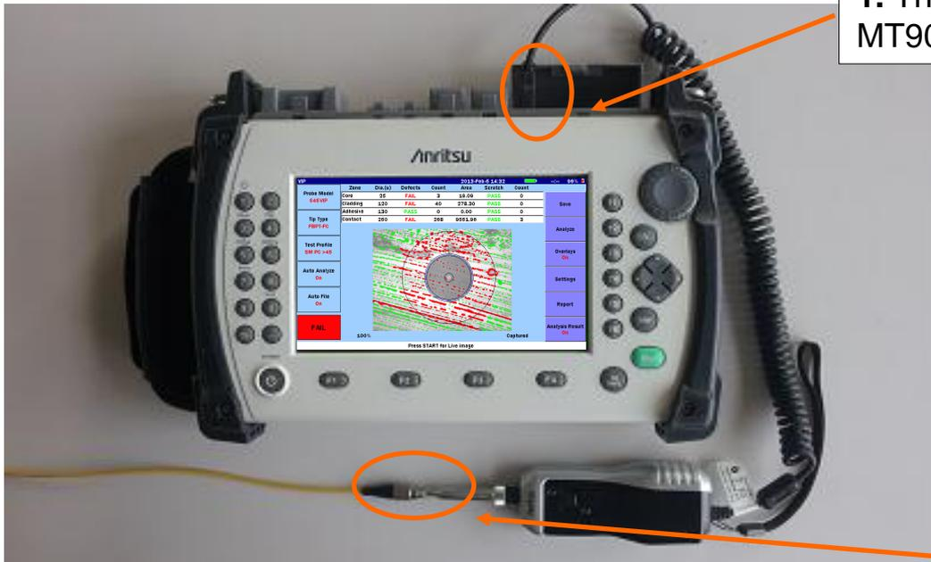
1. The VIP USB terminal is connected to the MT9083x2 series instrument's USB port.
