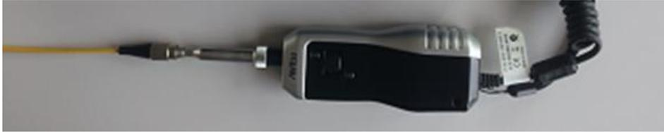
Tips are connected to the end of the VIP based on the shape of connector (adapter) to be connected. This unit comes standard with 7 types of tips.
