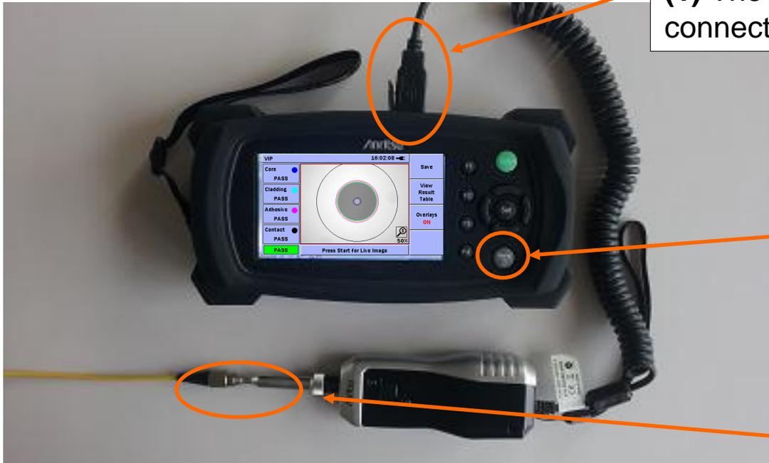
**(1)** The VIP USB terminal is connected to the MT9090A's USB port.
