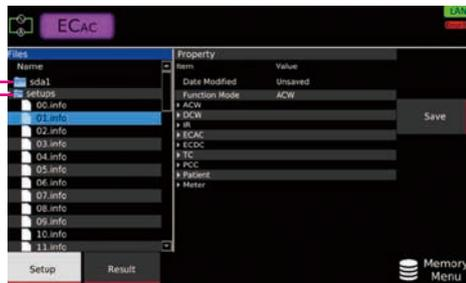
Testing conditions can be saved in 00-50 of "setups". (Total 51)
