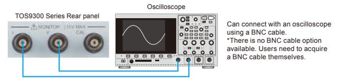
Can connect with an oscilloscope using a BNC cable.
