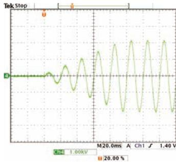
The rise time control feature allows you to gradually increase voltage to a set value while AC/DC hipot tests are conducted. Voltage rise times can be set from 0.1s to 200.0s at a resolution of 0.1s.
