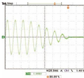
The fall time control feature allows you to gradually decrease the test voltage after a successful AC/DC hipot test. The voltage fall time can be set from 0s to 200s at a resolution of 0.1s. (OFF is also selectable).
