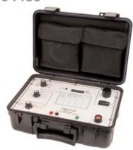
The PSD30-2AF is designed to calibrate and troubleshoot any DC capacitive fuel quantity system. The PSD30-2AF will perform the following functions:
