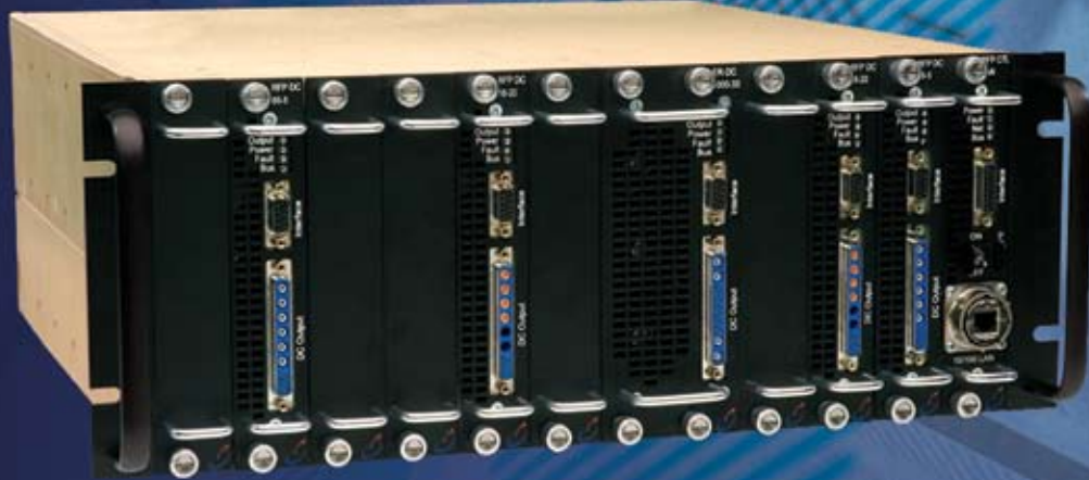
Modular Programmable Precision AC/DC/Loads Power System
